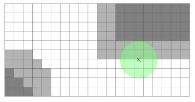
(It'd be nicer to do a more circular convolution, so that the sharp corner in the top-right gets smoothed to a more rounded corner, especially with large clearance values. That would be a self-contained enhancement and won't have any further consequences.)
