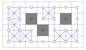
From any passable navcell, you can move to any horizontally/vertically adjacent passable navcell with cost 1. Also, you can move diagonally from any navcell (i, j) to  $(i \pm 1, j \pm 1)$  if those navcells, plus the adjacent navcells  $(i \pm 1, j \mp 1)$  and  $(i \mp 1, j \pm 1)$ , are all passable. Diagonal moves have cost  $\sqrt{2}$ .
