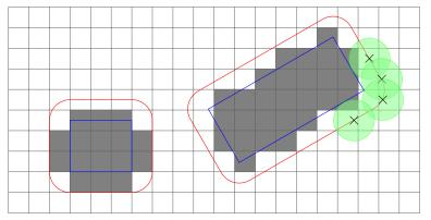
It is important that partially-obstructed navcells are still considered passable: when a unit is trying to move to a building (e.g. to attack it), it can always succesfully get within any distance d > c of the obstruction shape, without having to move illegally onto an impassable navcell.
